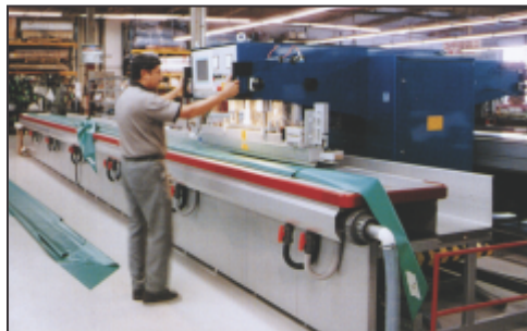
PTFE, PVC and HDPE membranes are fabricated in-house using state-of-the-art heat-sealing, RF welders and industrial sewing machines.
