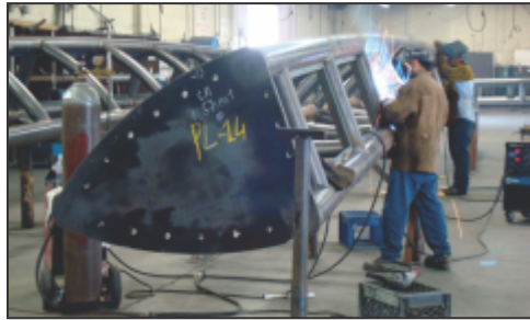
Metal structures are custom designed and manufactured in-house by our certified welders. Los Angeles Approved Fabricators License #1716.
